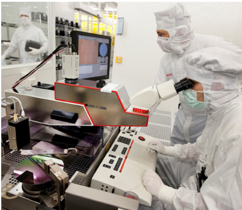
Swabian efficiency: micromechanical components are created in sterile clean rooms
